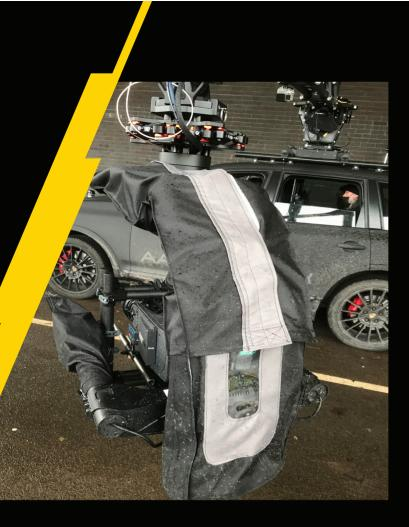
The FOG System over-rides the standard MEMS sensors on the standard XL head and turns our Movi XL into a completely different animal. It stops pan drift, neutralises high-frequency vibration and disturbance making it reliably stable at high speed and for use with longer lenses. In terms of operator response and overall performance, the FOG makes our Movi XL a match for heads renting for twice the price. Type 'Movi XL FOG' into Youtube for a quick two minute video.
